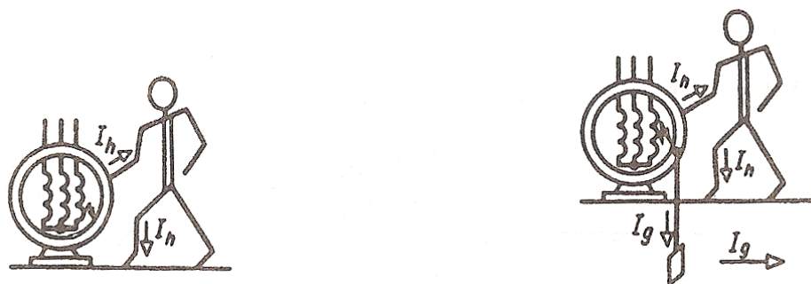
a) Contact with an ungrounded motor frame
