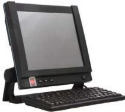
The Message Terminal has a touch-screen for operating the system. You can also use the keyboard, which is mandatory in GMDSS systems.
