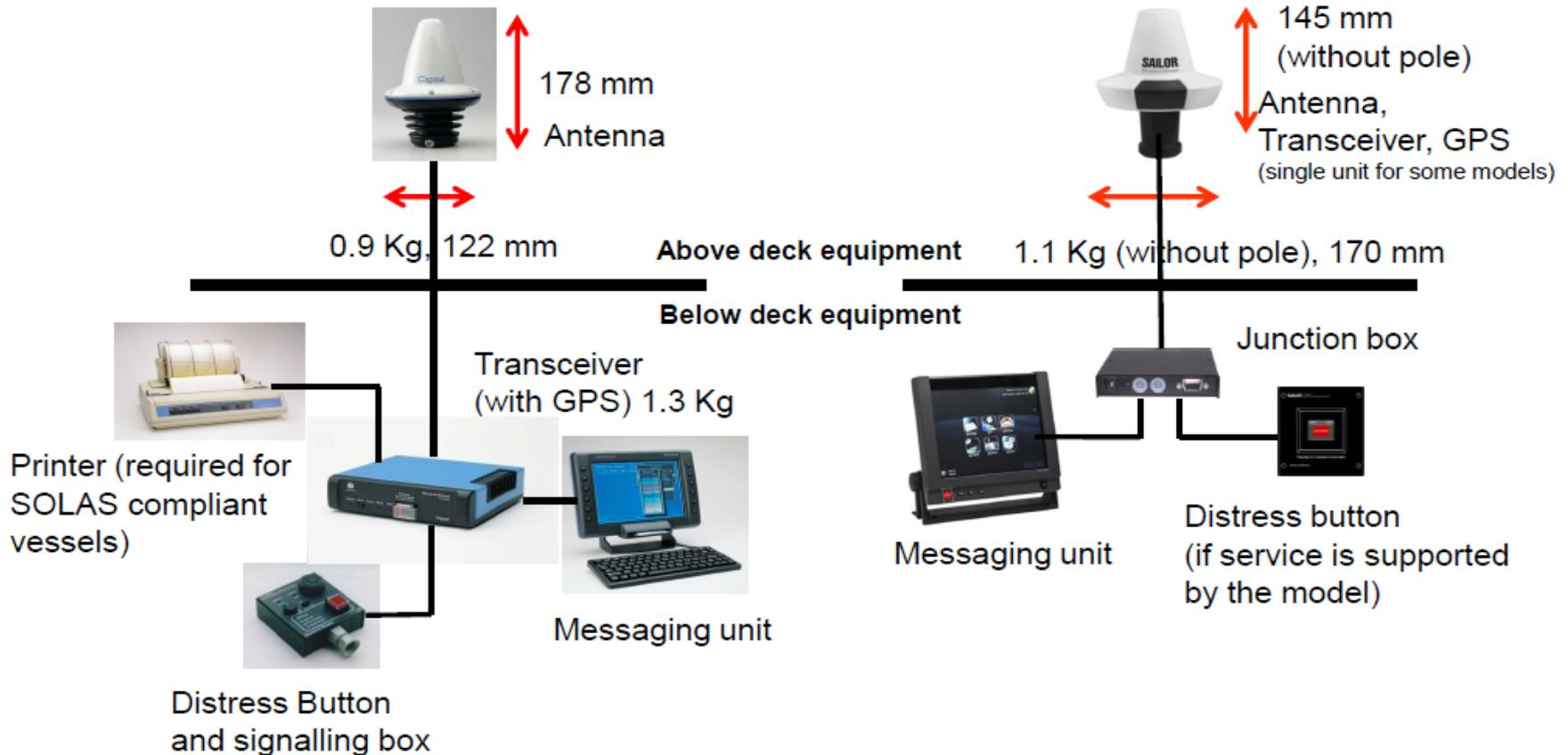
**Note: No power supply is shown for both configurations**
